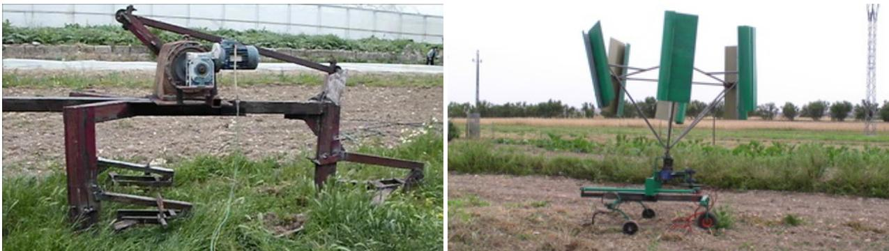
**Figure 11:** *Left: UTOPUS for deeper tillage (20 cm), March 2012. Right: Wind powered design, June 2012.*
