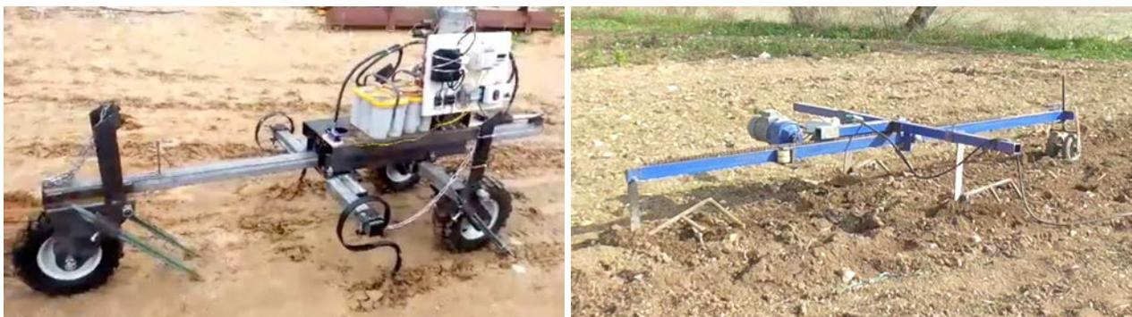
**Figure 12:** *Left: Hydraulic drive train, April 2014. Right: Simplified electric design, November 2014.*
