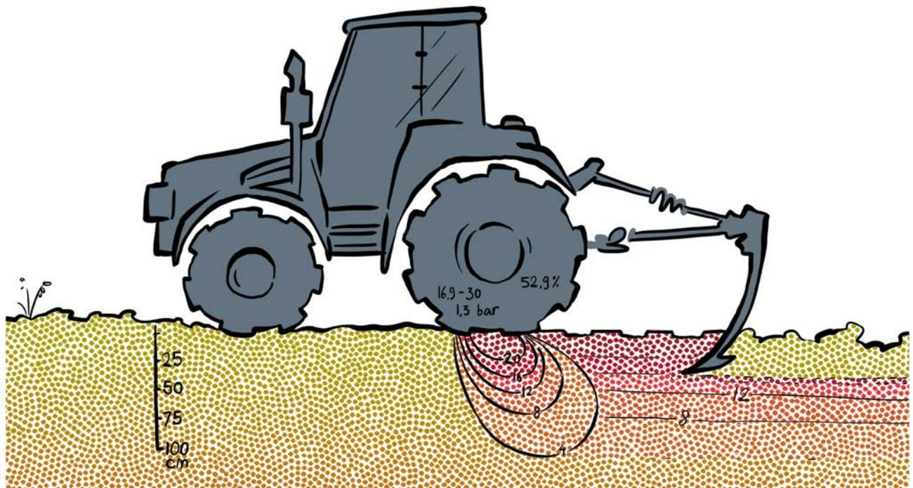
**Fig. 1.** The main axis of the pressure bulb under a tractor tire extends diagonally into the ground and compacts the soil below the depth of tillage (Söhne and Bolling, 1981).
