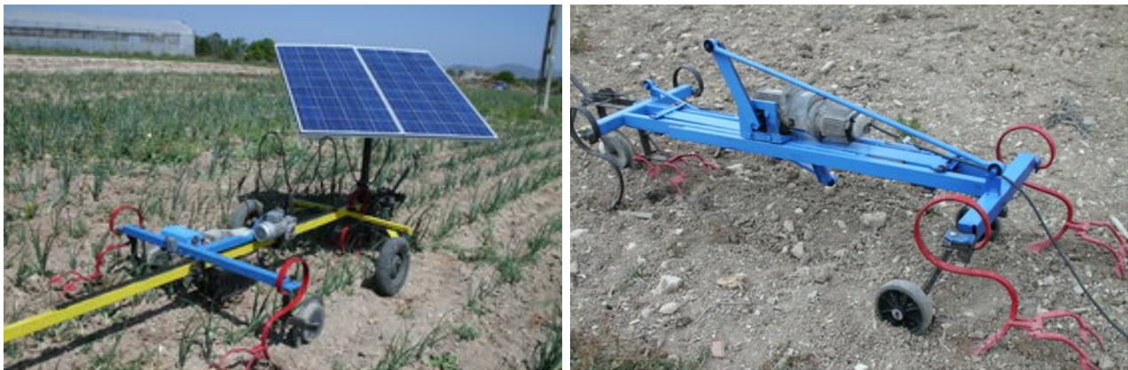
**Figure 10:** *Left: Improved design of June 2011. Right: New drive train, October 2011.*
