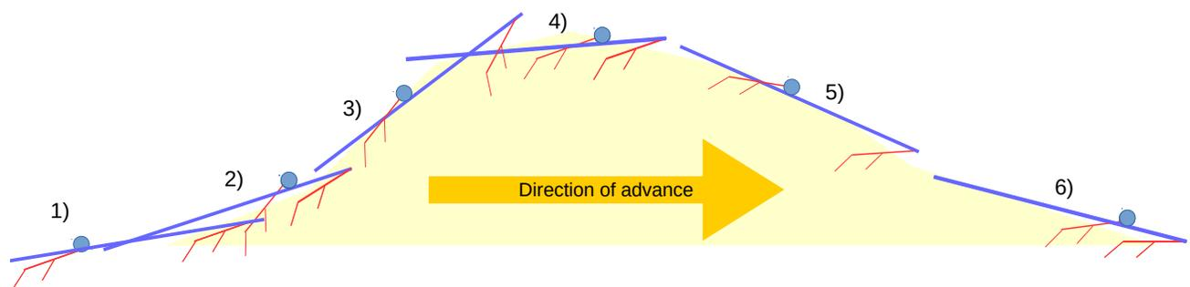
**Fig. 6.** Schematic drawing of UTOPUS mound climbing maneuver. **1)** UTOPUS approaches the mound and initiates the climb. **2)** UTOPUS passes the concavity at the base. **3)** UTOPUS climbs the side of the mound in a steady line. **4)** When the front end of UTOPUS extends beyond the surface, UTOPUS swings into a horizontal position. **5)** UTOPUS descends safely in a controlled descend. **6)** At the base UTOPUS passes another concavity.
