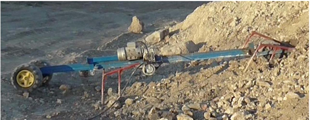
**Fig. 8:** As UTOPUS begins to climb, the distance between the shaft and the ground increases at the concavity, such that the crampons have less contact with the ground.
