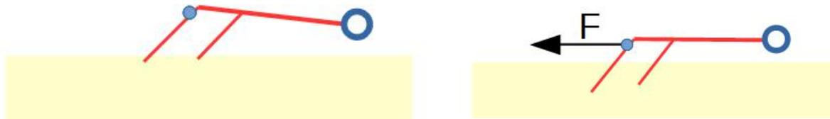
**Fig. 5.** Crampon design. The hinge at the back of the frame is indicated by a blue circle. **Left:** The crampon before entering the ground. **Right:** The crampon anchored in the ground, resisting the drawbar pull  $F$ .
