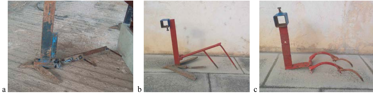
Figure 2. Empirical crampon designs. In each photo, there is a vertical shaft which connects the crampon to its implement frame. At the base of the shaft there is a horizontal hinge to which the crampons are connected, allowing them to swing up and down. The straight crampons in (a) and (b) penetrate soil to a depth of 10cm and 20cm respectively, the curved crampons in (c) penetrates to about 5cm. (a) and (b) also have a tillage implement (a sweep) connected to the base.
